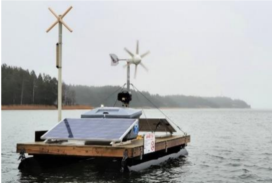
Figure 3. Raft carrying an ADD unit and outfitted with solar panels and a wind generator for charging the batteries. Photo: Esa Lehtonen
