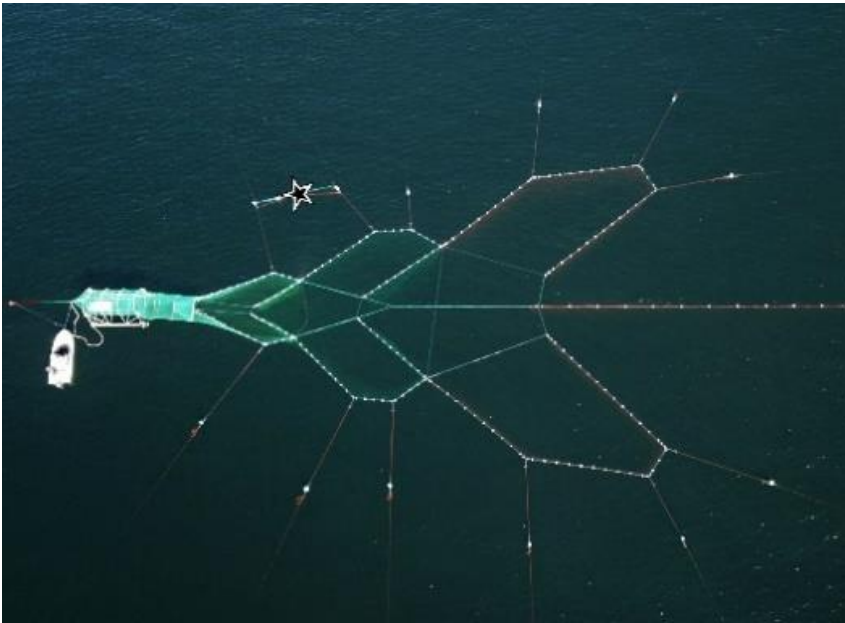
Figure 2. Aerial view of a pontoon trap with the chamber, intermediate funnels and wings. Only a part of the leader net is shown. The seal deterrent is marked with a star symbol. Photo: Esa Lehtonen
