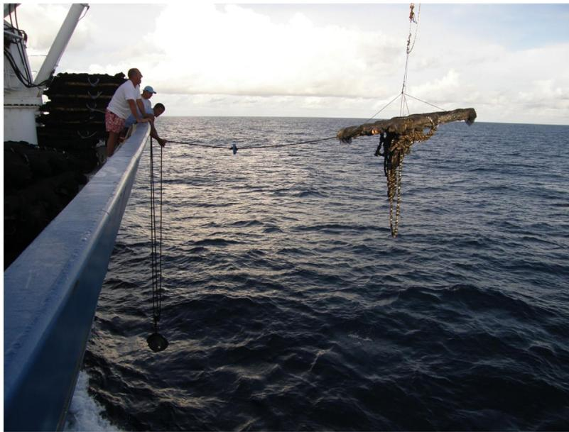
Fig. 1. Deployment of DFAD structure with an echo-sounder buoy from a purse seiner.
